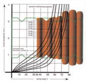
Pur-Cell is a cellular foam that is excellent for shock absorption of light to medium loads at high frequencies. A cellular Vulkollan piece is able to be compressed up to 70% of its original height with minimal permanent set. Pur-Cell parts are available in custom molded shapes, sheet, rod, and tube.
