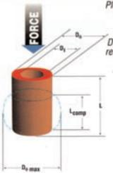
Plei-Tech® polyurethanes, based upon NDI, PPDI, and TDI are typically used in shock absorbing applications. Depending upon the application requirements, these compounds are varied in configuration, durometer and chemical make up to offer the best performance.
